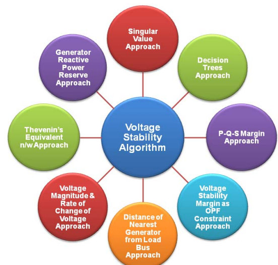
Fig. 1 Different Approaches for Real Time Voltage Stability Analysis using Synchrophasors
